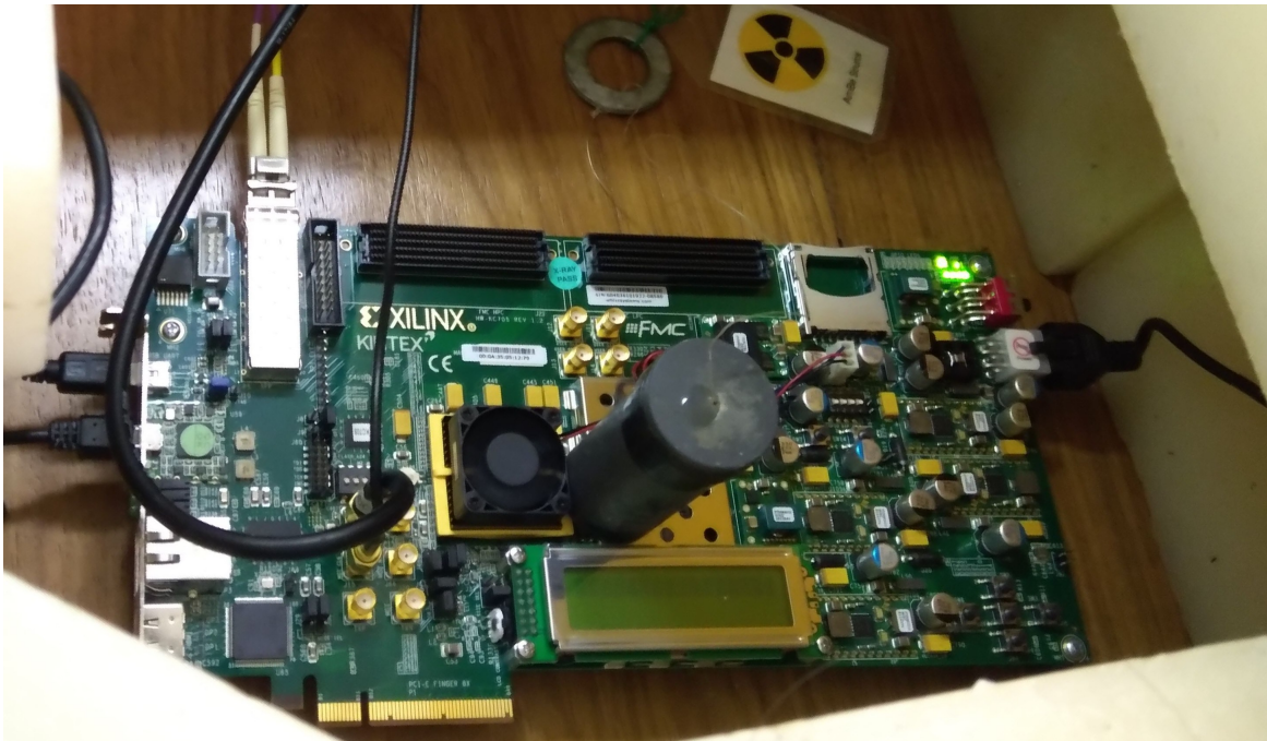
Figure 4.5: AmBe source positioned on the FPGA board.
