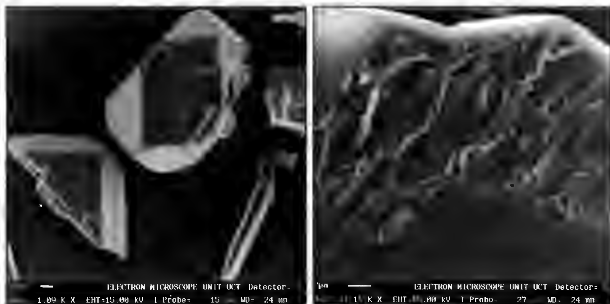
Figure 5.26. Secondary electron images of mineral surface etching on Kopoasfontein apophyllite reacted for four weeks in HCl/NaCl solution of pH 3.
