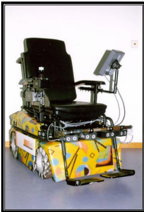
Figure A-12: Omnidirectional wheelchair developed by Hoyer et al at the University of Hagen [10]
