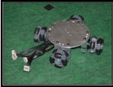
Figure A-16: Cornell's four wheel omnidirectional robot introduced in 2001 [18]
