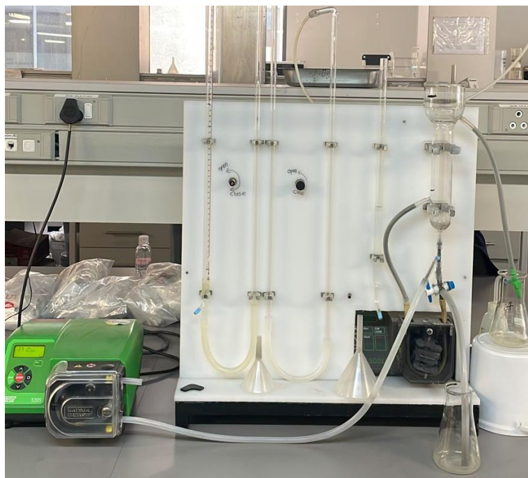
Figure 3.4 UCT microflotation rig with the pump used to supply a steady airflow at a rate of 8 ml/minute
