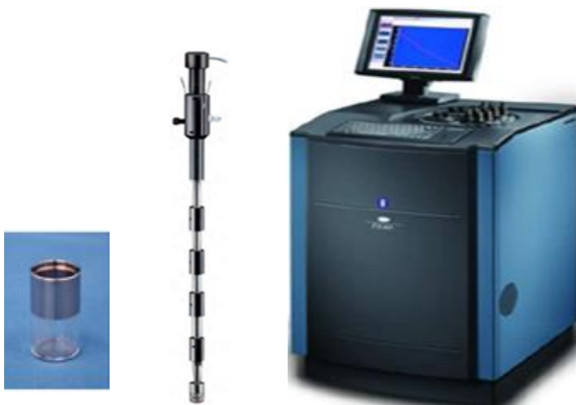
Figure 3.9 TAM III Isothermal Titration Microcalorimeter machine with the loaded shaft and the sample ampoule
