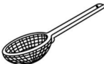
Figure 22: Float and sink apparatus - wire mesh strainer
