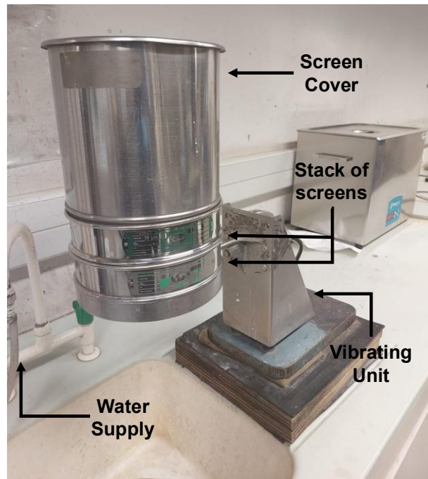
Figure 19: Wet screening apparatus with stacked sieves
