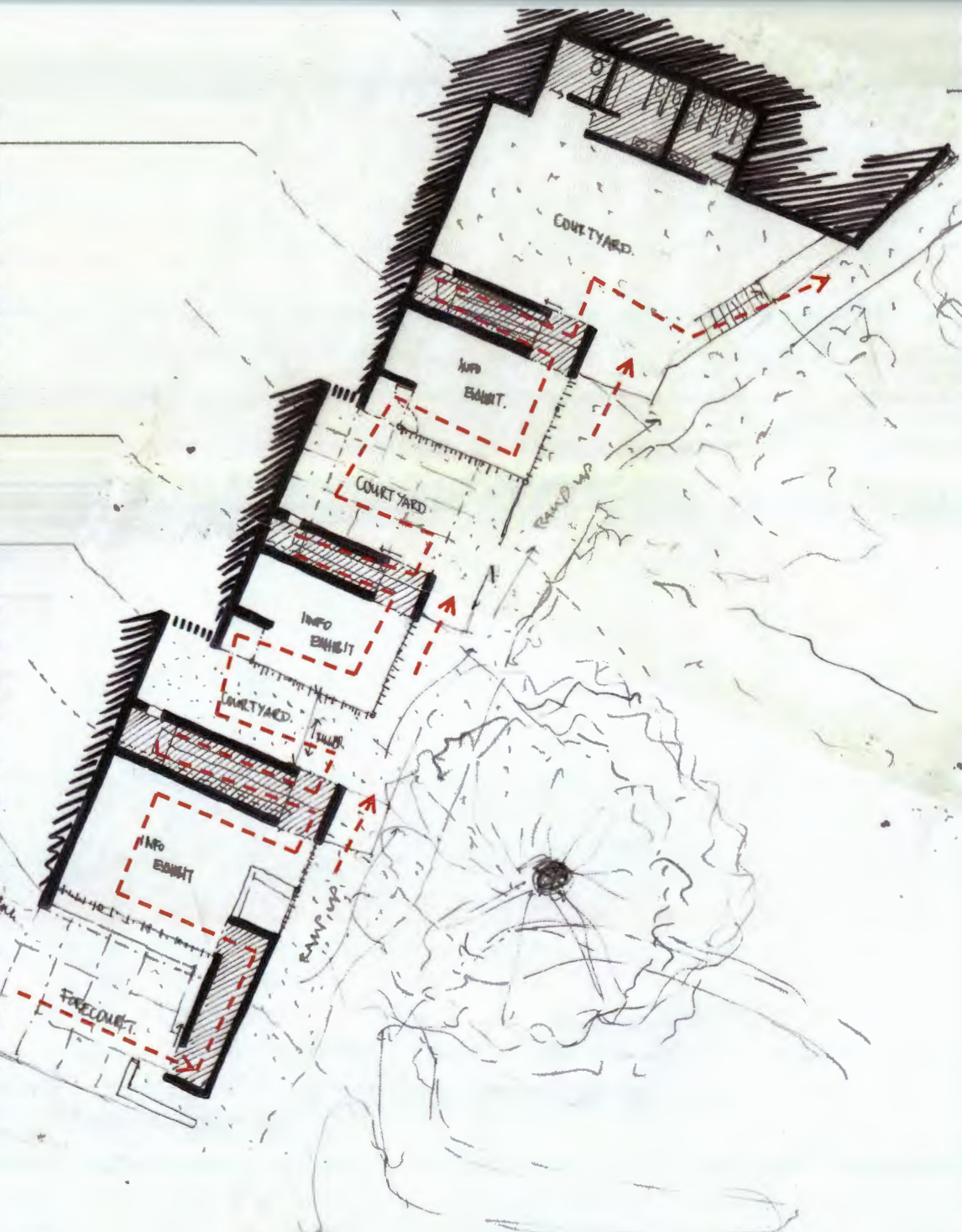
Fig. 49 Plan of Visitor's Center Exploration of dark and light spaces; thick walls; open protected courtyards, occurring on a movement route into site.
