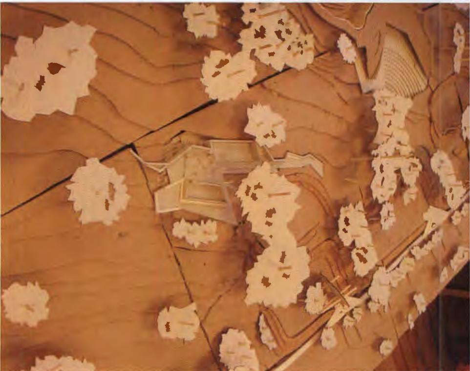
Fig. 52 Early working model Visitor's Center: working with a route along contour, as opposed to up slope into site
