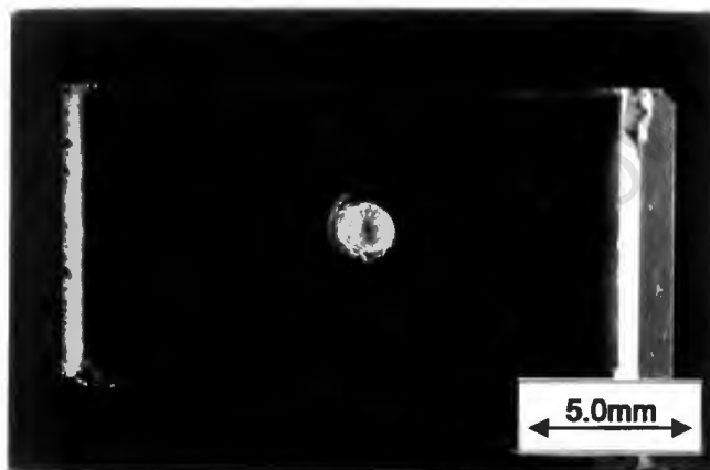
Figure 17. Top view of a test block impacted in the centre at an energy of 1J
