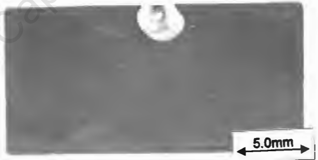
d) G10: 10%Co, 2.0 \mu m Grain Size
