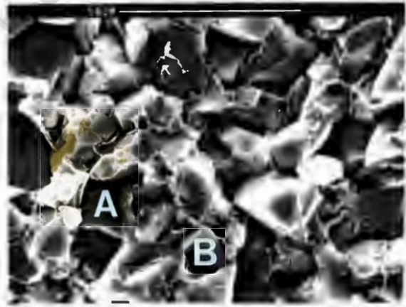
36.d) G10: 10%Co, 2.0 \mu m Grain Size
