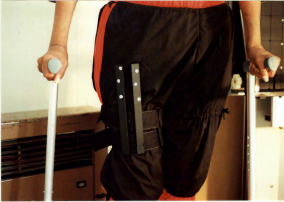
Figure 5.6. The black cover garment and external markers used for the patient studies.
