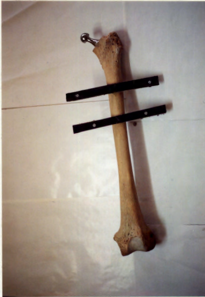
Figure 5.4. One of the dry bone specimens showing the implanted femoral component and the positions of the external markers
