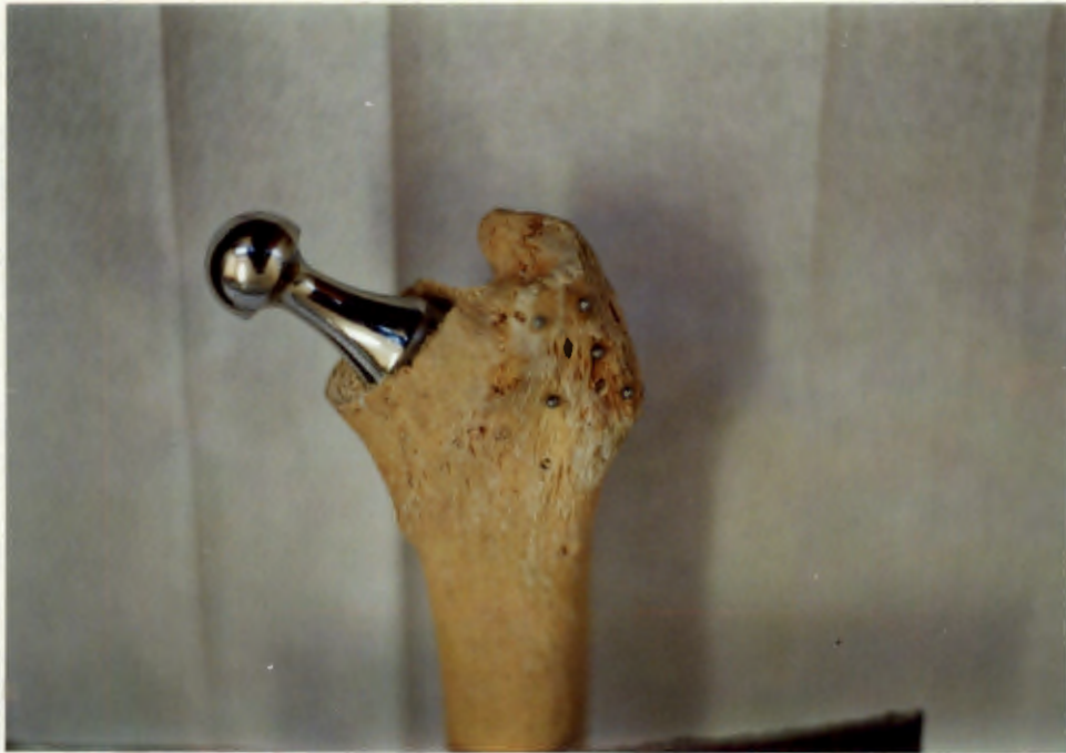
Figure 5.5. The bone specimen with the accuracy beads glued in position.
