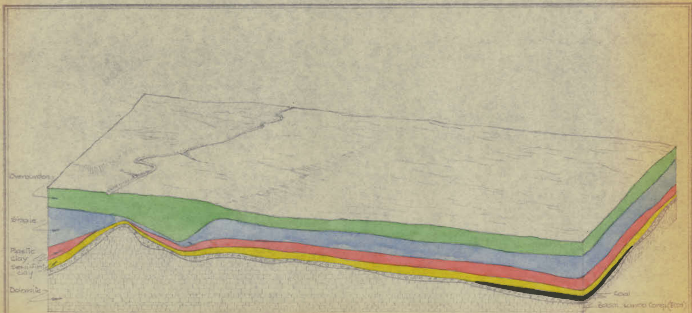
BLOCK DIAGRAM SHOWING RELATION OF REFRACTORY CLAY SEAMS (ECCA) AND UNDERLYING ROCKS SPRINGS AREA Vertical Scale Exaggerated
