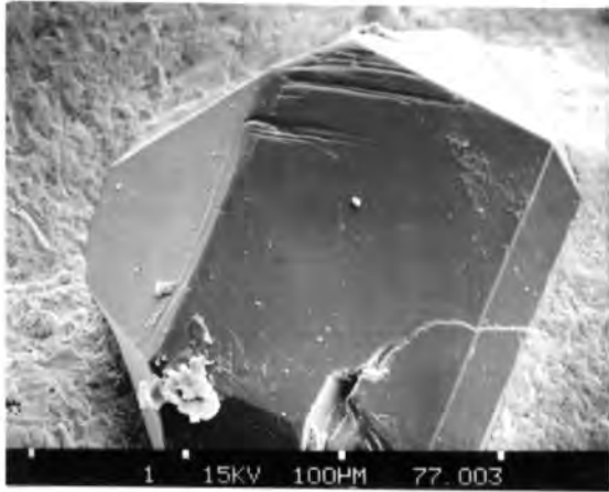
(a) : Type 1a - grooving and rounding on the apex of a stone with a fracture
