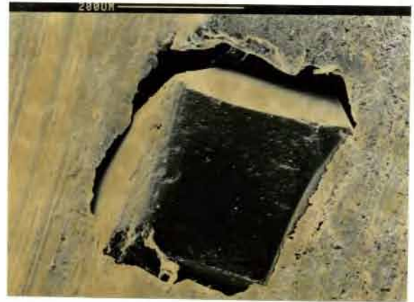
(b) : Type 4b - stone forced into matrix : Jaspilite
