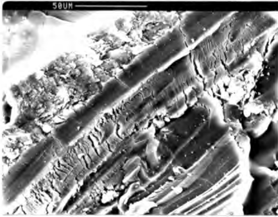
(a) : Sintered flake showing plastic grooving
