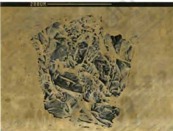
(e) : Type 4a - stone fractured until flush with the matrix : Quartz
