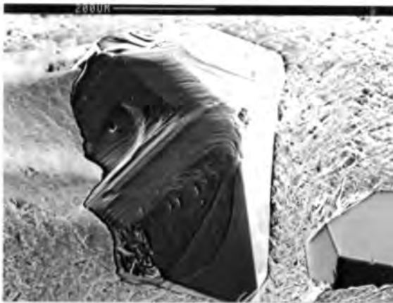
(c) : 30/40 mesh : Type 1b wear with transverse steps on lower diagonal edge
