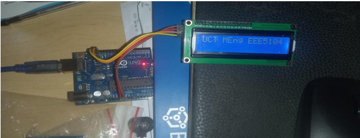
Fig 2. 15: Testing LCD Module
