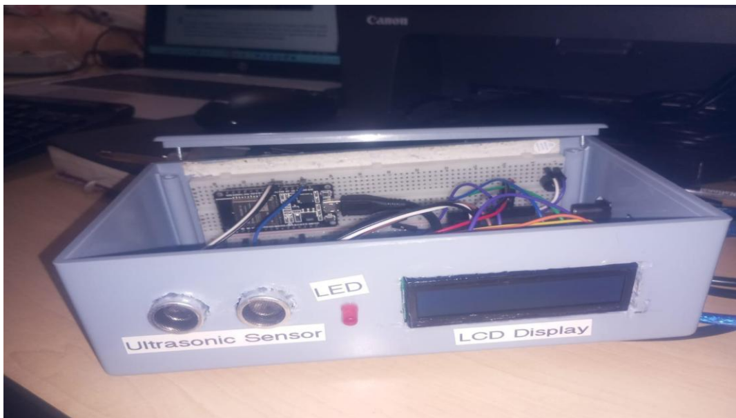
Fig 3.5: Ultrasonic Sensor-based Prototype – Front-view
