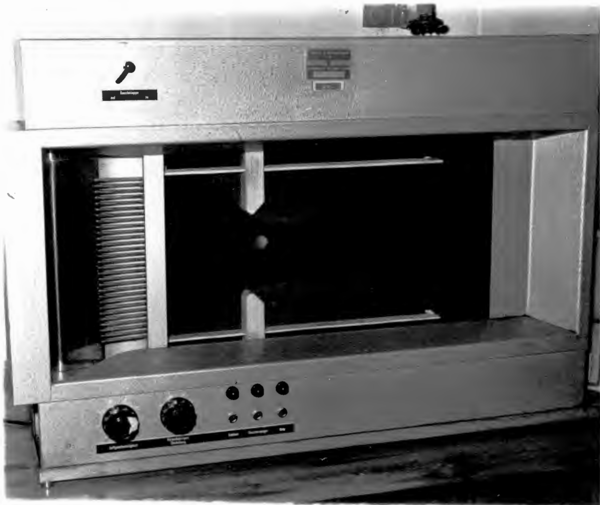
Fig.34. Smoke Tunnel Used for Flow Visualization.
