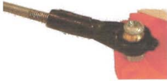
Figure 25: Close up of ball and socket joint.
