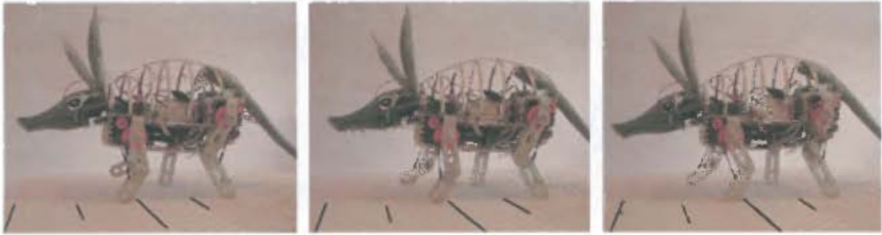
Figure 52b: Walking sequence part two. The back right leg is then driven further and the other legs adjusted so that the weight is taken off the front right leg. This leg is then tucked up and brought through, before being stretched out to the front. The other legs are then adjusted so that the weight tips onto the extended front right leg, and this frees up the rear left leg.
