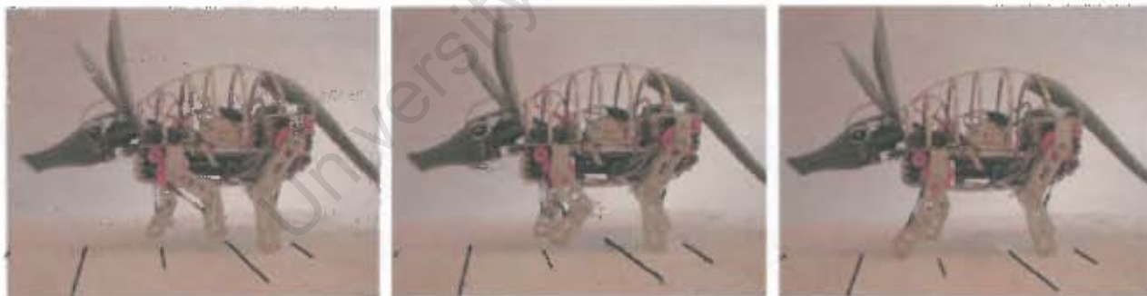
Figure 52d: Walking sequence part four. As the front left is brought through and stretched out to the front, the other legs are adjusted so that the weight tips onto the front left leg, freeing up the rear right.
