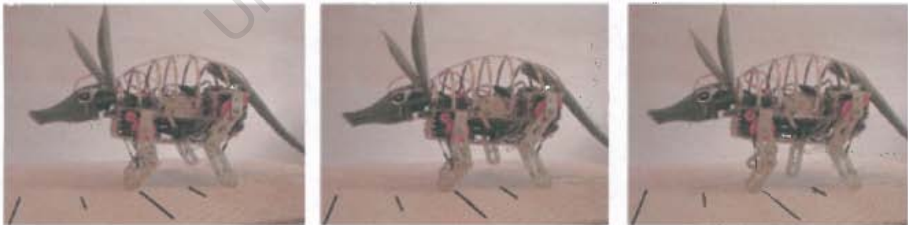
Figure 52a: walking sequence part one. First, the legs are shifted so that most of the weight is over the front legs. The front left leg is then dipped slightly, and this frees up the back right leg. The back right leg is then tucked up and brought forward, before being straightened and placed on the ground just behind the front right foot.
