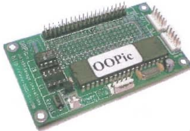
Figure 12: OOPic microcontroller board
