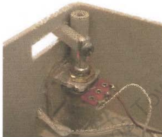
Figure 45: Potentiometer used to control the upper eyelids
