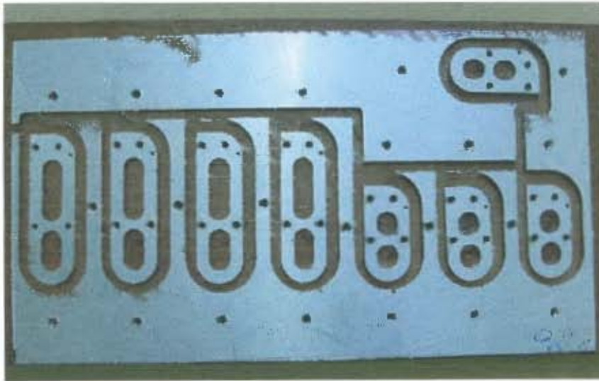
Figure 22: Photo of the CNC machined aluminium leg plates.
