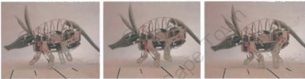
Figure 52c: Walking sequence part three. The rear left is then tucked up and brought forward to be placed behind the front left foot. As was the case with the rear right leg earlier, the rear left is used to take the weight off the front left (the other legs are adjusted to help this too), and the front left is then free to be tucked up and brought forward.
