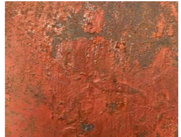
Fig. 21. Patina and rust of salvaged metal piece
