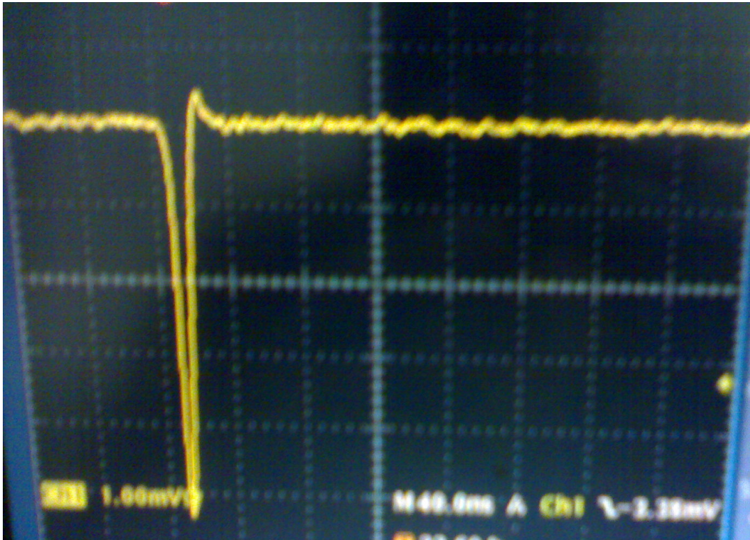
Figure 4:35. Signals obtained with the redesigned recoil detector.
