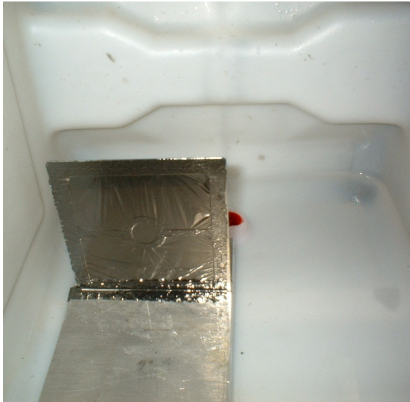
Figure B:4. The carbon foil fully mounted on a frame.
