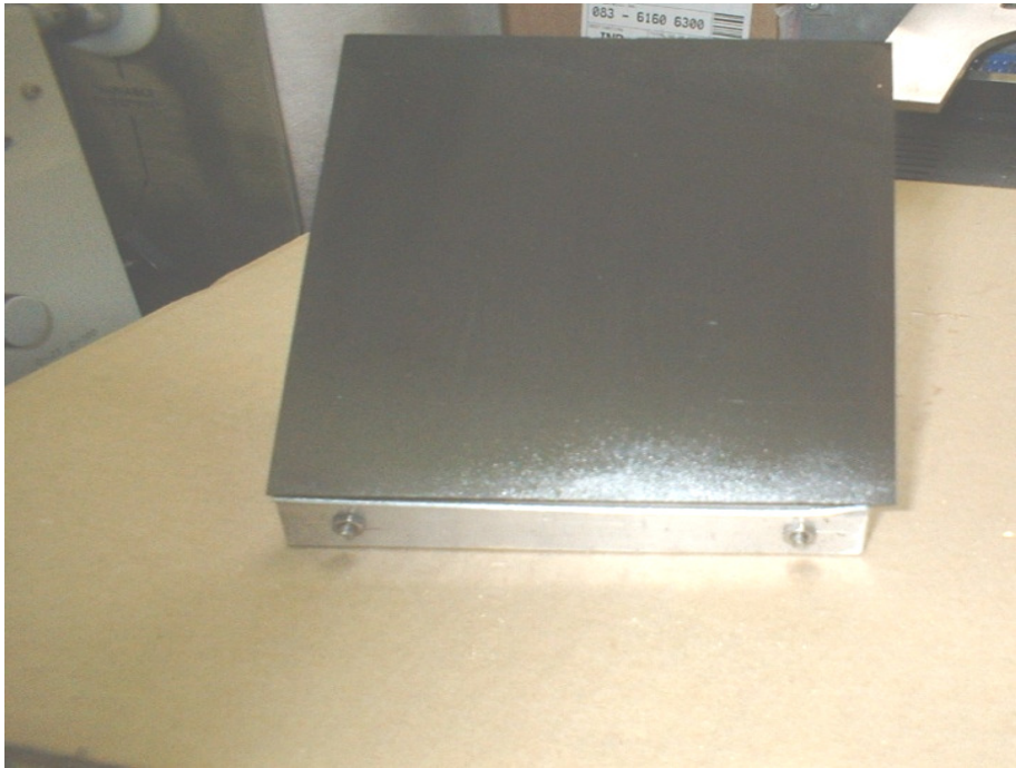
Figure B:1. Carbon coated glass on a 45° aluminum stand.
