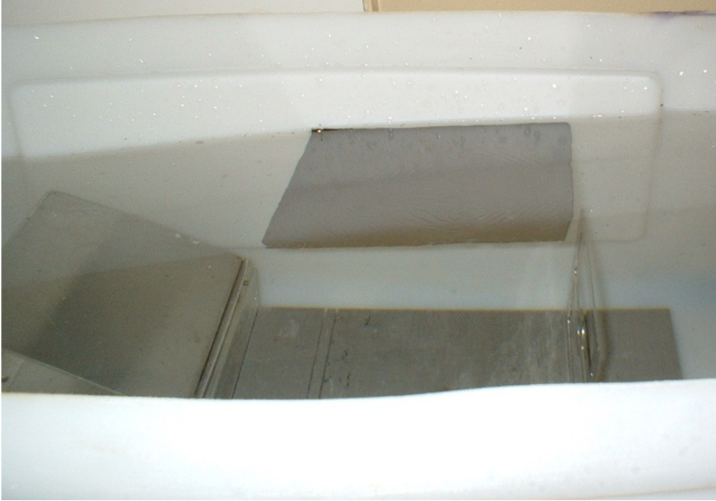
Figure B:2. Carbon foil floating in the tank after the water level has risen above the frame. The foil has floated free of the substrate. The foil is then moved gently until one edge lies above the frame. The water is then moved slowly out of the tank.
