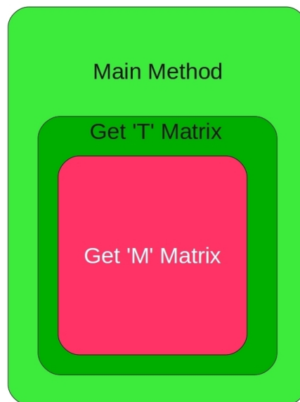
(b) Visualisation of the percentage of total time spent in the functions of interest. The section of code to be implemented in reconfigurable hardware is highlighted in red. It represents 61% of the T calculation function, which accounts for approximately half of the total running time. The section to be offloaded to the FPGA is thus 32% of the complete tracking problem.
