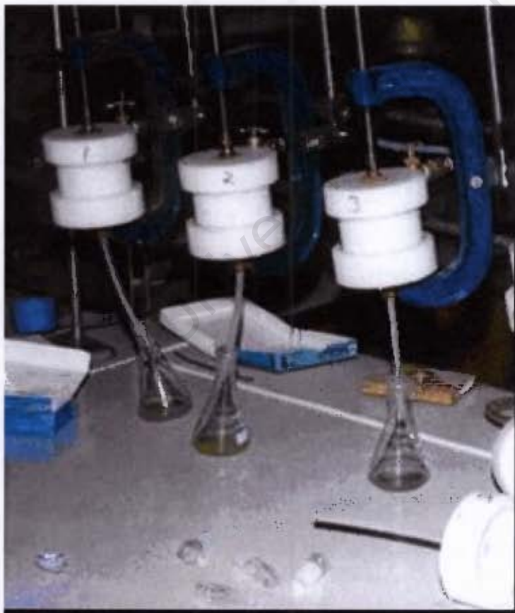
Figure 2.4 Reeburgh Teflon squeezing apparatus (Reeburgh, 1967).
