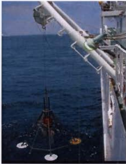
Figure 2.2: Multicorer device deployed over the side of the RV Welwitschia during a sampling cruise.
