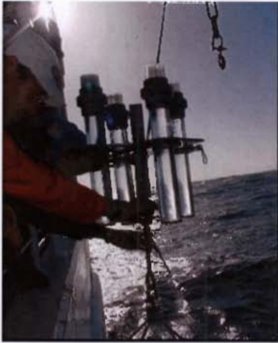
Figure 2.5 Retrieval of sediment traps deployed at Station A.
