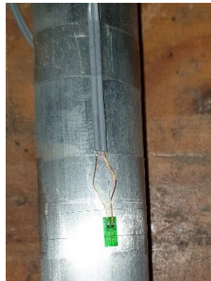
Figure 28 : A photograph showing the Strain Gauge mounted on the tubular structure [59]
