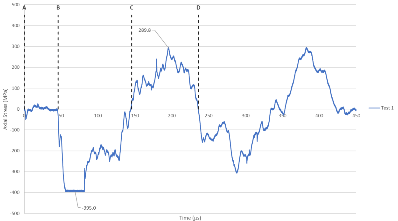
Figure 50 : The graph of stress history obtained from blast testing of Stepped tube with Deformable witness plate.
