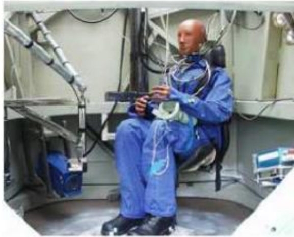
Figure 20 : An image showing Test Rig for Occupant Safety Systems (TROSS) set up with a Hybrid III surrogate [41]
