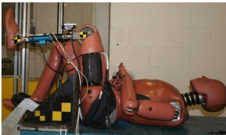
Figure 21 : The Linear impactor test set up[47]
