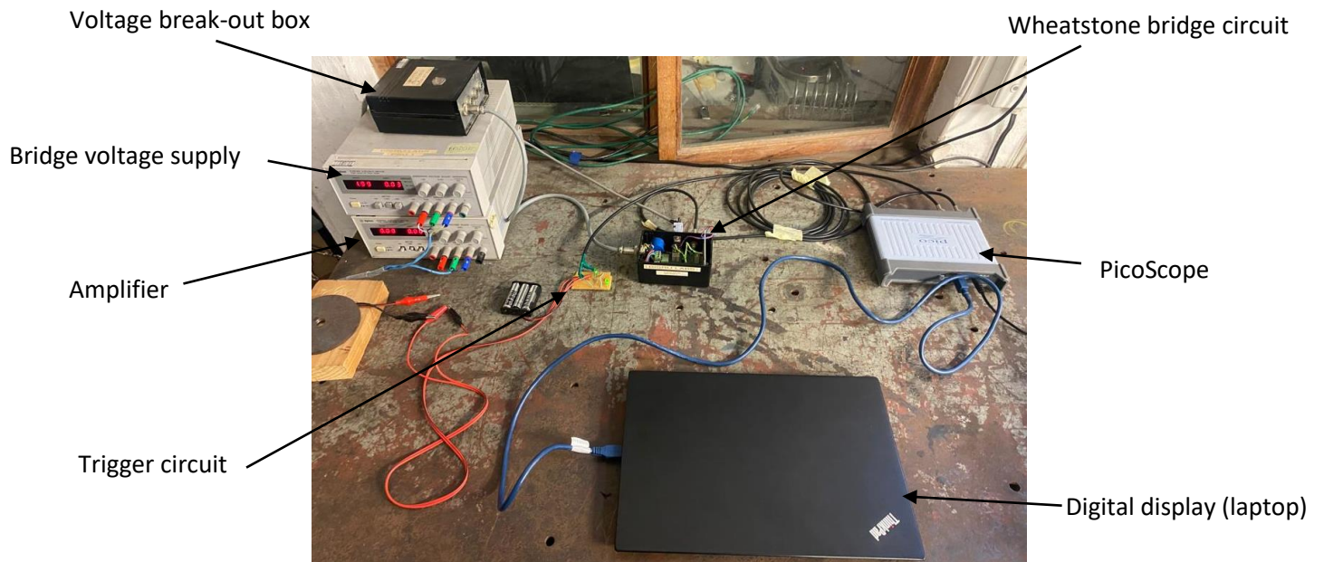
Figure 37 : A photograph of the data acquisition instruments set up used to capture the response of the tubular structure to blast loading.
