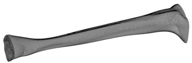
b) 3D Finite Element Tibia
