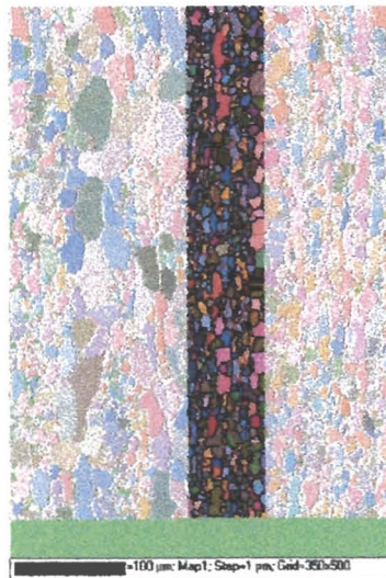
Figure 33. Calculating relative yield strengths in different grain size bands. Achieved by isolating grain size bands, measuring their grain size and calculating yield strength from Hall-Petch relation.
