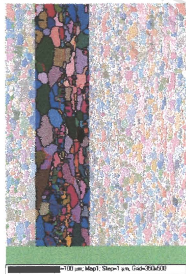
Figure 33. Calculating relative yield strengths in different grain size bands. Achieved by isolating grain size bands, measuring their grain size and calculating yield strength from Hall-Petch relation.
