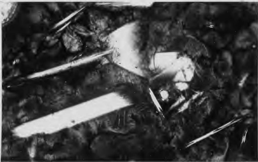
Figure 7 c. Zone 5. This illustrates the coalesced plagioclase spherulites comprising the groundmass. Also visible are needle like plagioclase microlites and quench olivine. 100 X magnification. Field of view = 1.45 mm. From AG32-3-113 (Group B).
