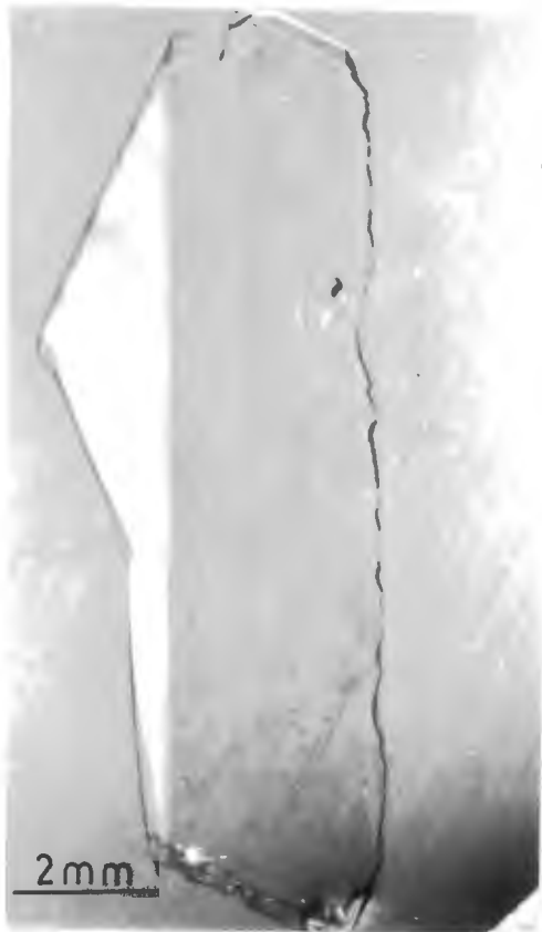
Fig.8.2 Optical micrograph of a basal section which has been annealed for 45 min. at 900K. A milky band on the L.H.S. is apparent.
