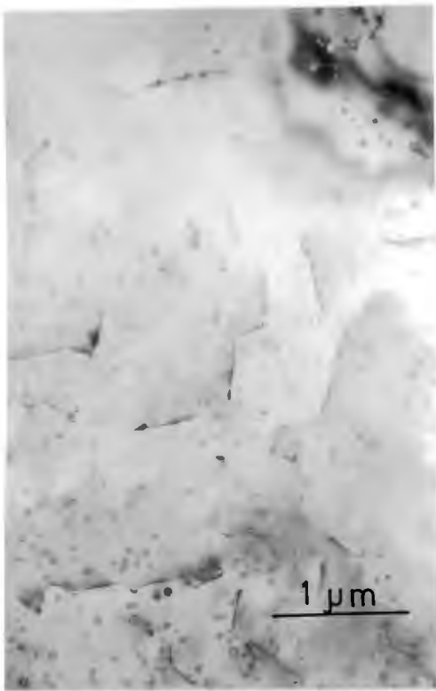
Fig.8.9 High voltage electron micrograph of a 'wet' band after an anneal at 1100K for 38 hrs. A network of dislocations and thin hexagonal precipitates are present.
