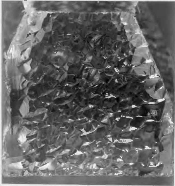
Fig.2.8 Typical Z-growth synthetic quartz, showing the rough face, or 'cobble texture'.
