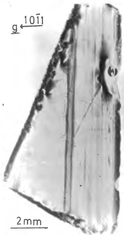
Fig.8.4 X-ray topograph of above basal section prior to annealing.
