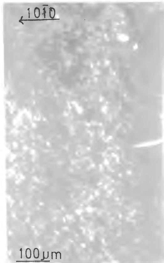
Fig.8.3 Optical micrograph taken close to the edge of the milky band of fig.8.2. The defects can be resolved and lie on (10\bar{1}0) planes.
