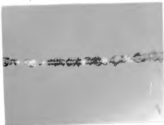
Fig.10.46 Scratches made at room temperature in moist laboratory air. (sharp pyramid).
