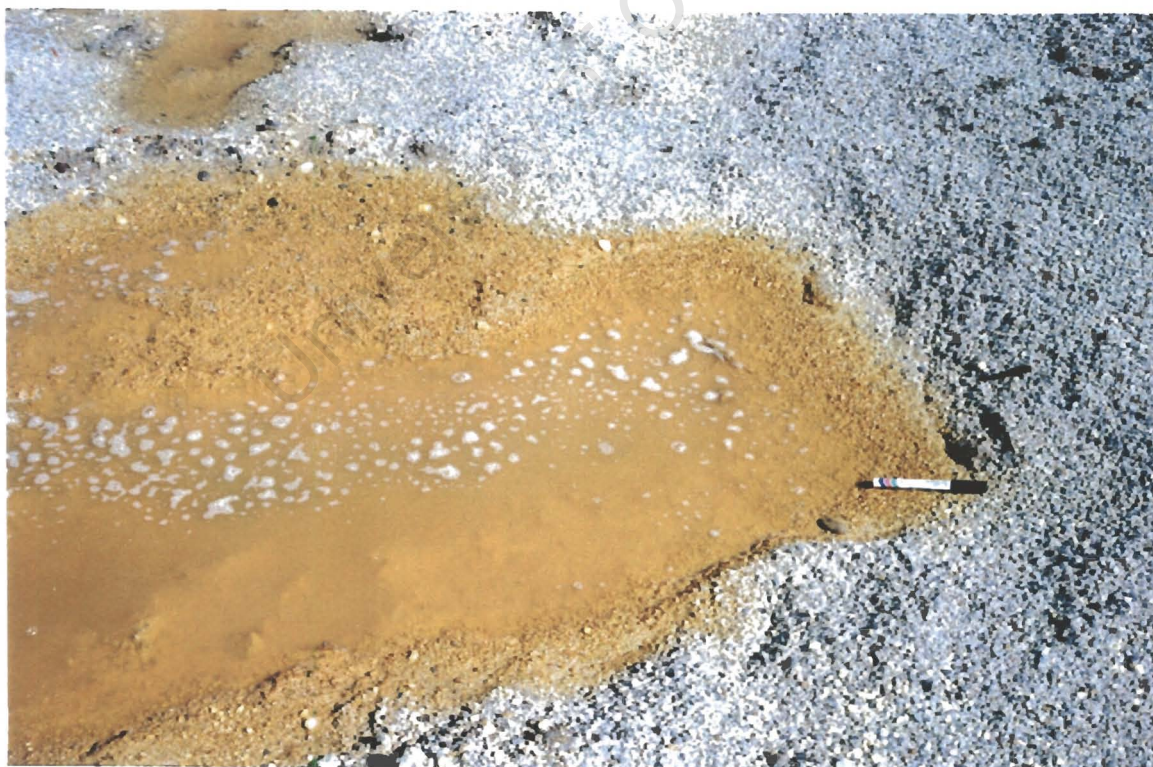
B. Limed water (pH 3.8) with Fe precipitates forming on the surface of limestone grains.
