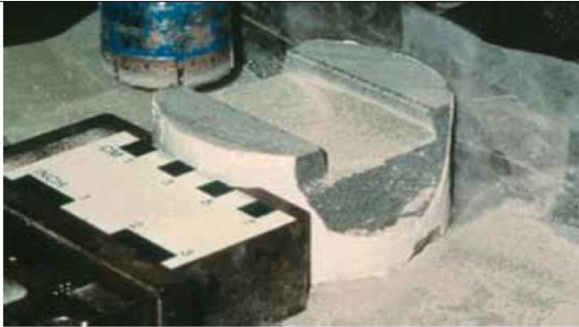
Figure 5.2: Milling ASTM C1556 specimen in 1 mm steps (Stephen et al., 2010)
