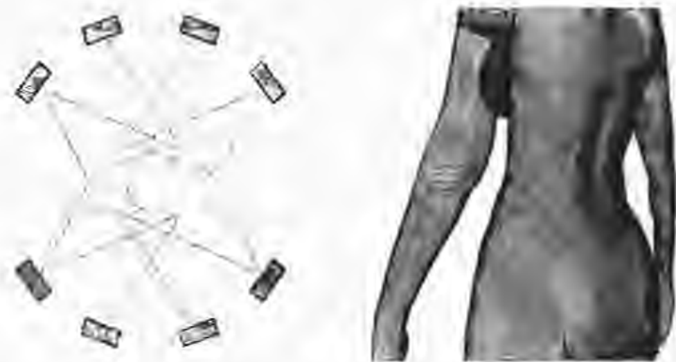
Figure 2.3 Scan configuration (left) and quadmesh representation for skin surface (right) (Wells et al 2000)
