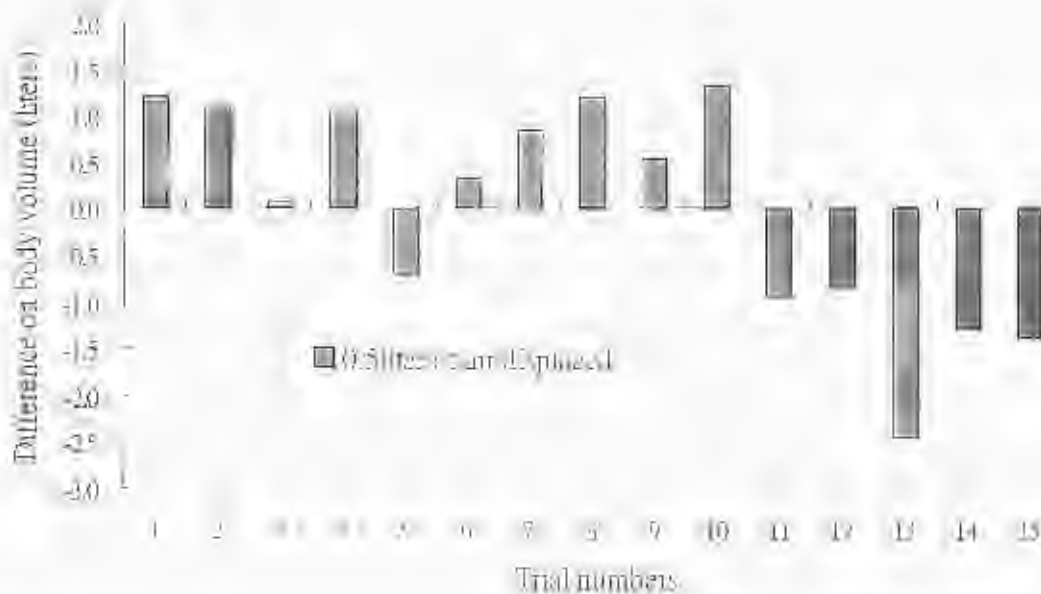
Figure 8.5 calculated body volume for 15 trials on the same subject using a single chamber driven by a motor driven pump
