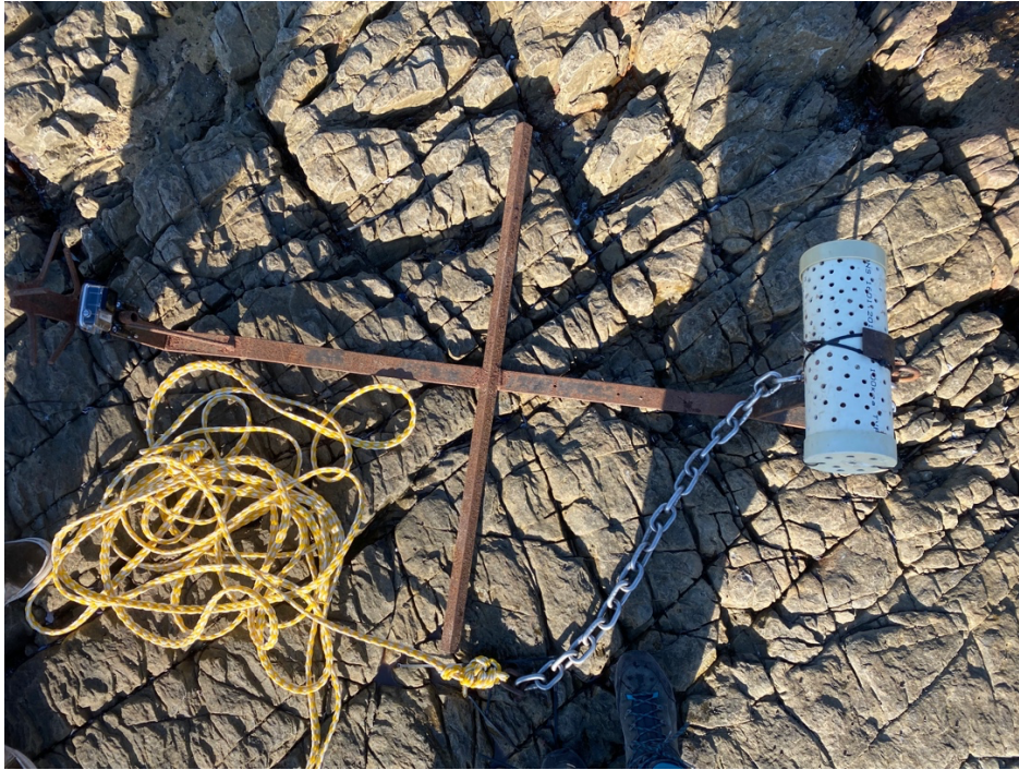
Figure 12: Baited remote underwater video equipment with the camera facing the bait canister, attached to a steel rig.
