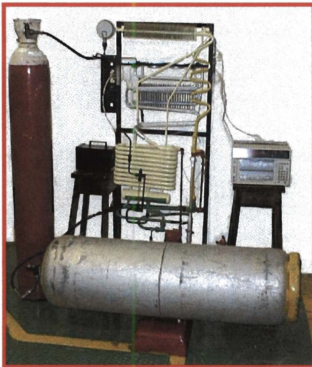
Figure 4.6 Charging of ammonia and hydrogen
