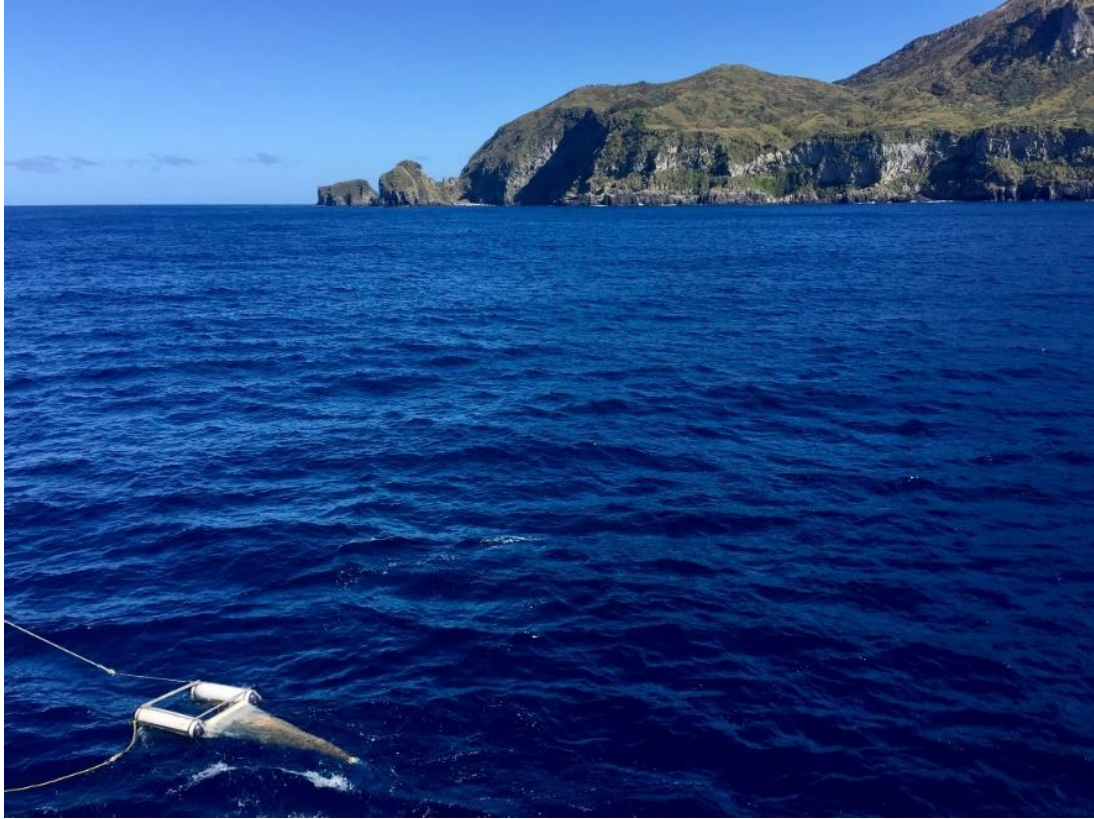
Fig. 1.4 A neuston net being slowly trawled alongside the S.A. Agulhas II research vessel to sample floating meso- and microplastics off Gough Island, central South Atlantic Ocean in 2019 (photo Vonica Perold).
