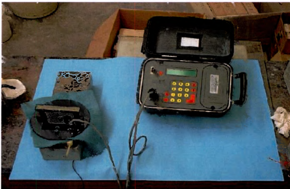
Figure 4.13 Typical Gecor measurements using sensor A on test specimens
