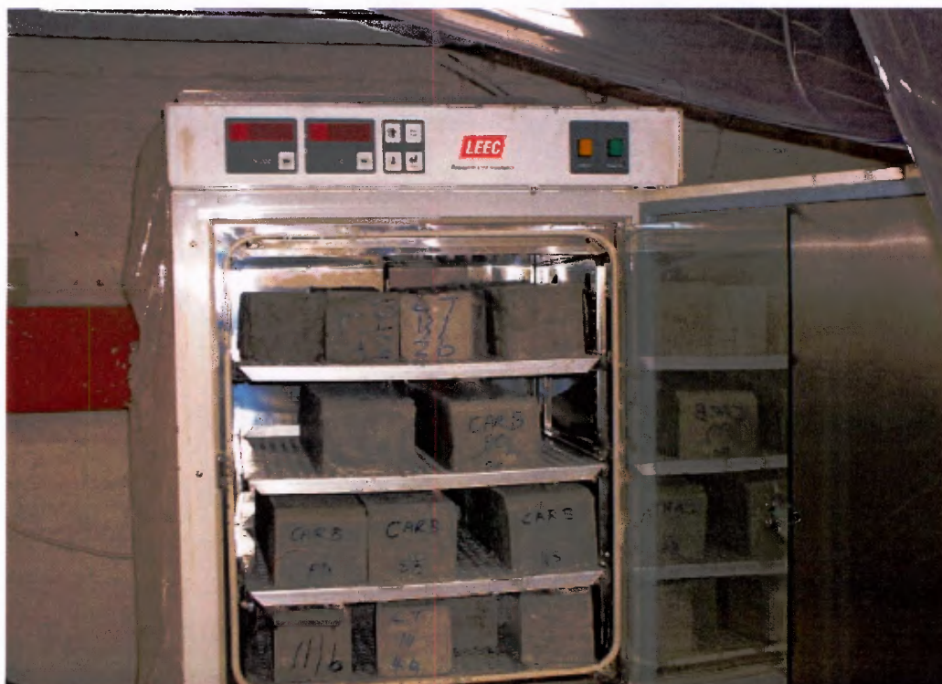
Figure 4.7: Set up of test specimens in carbonation chamber
