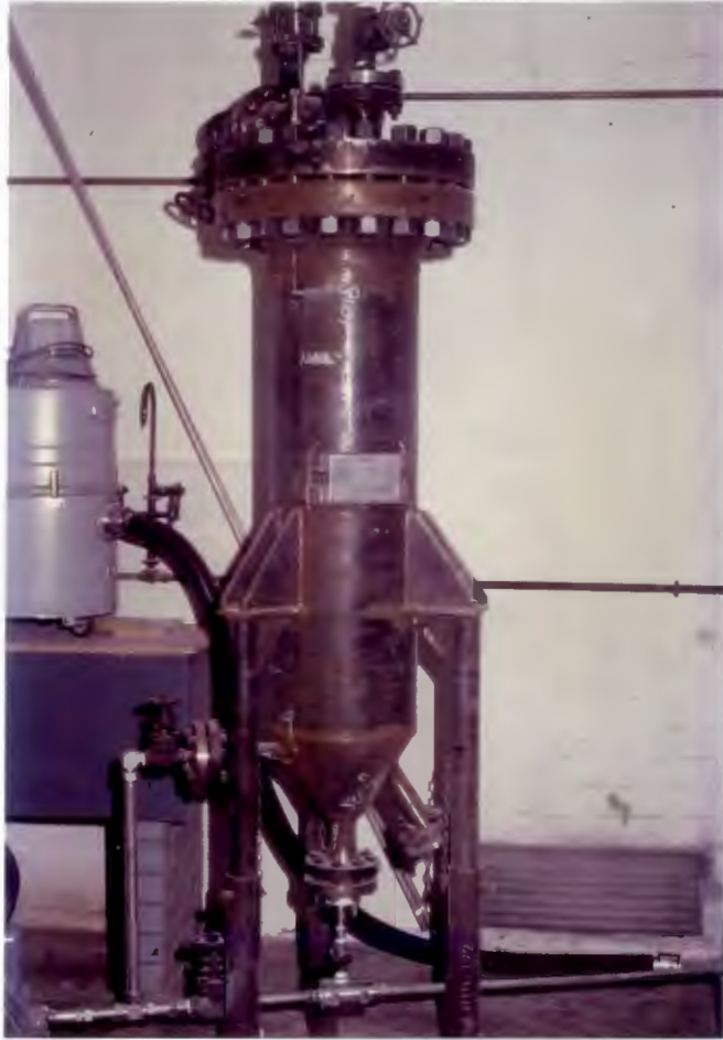
FIG : 3.4 Experimental ash hopper (without insulation).
