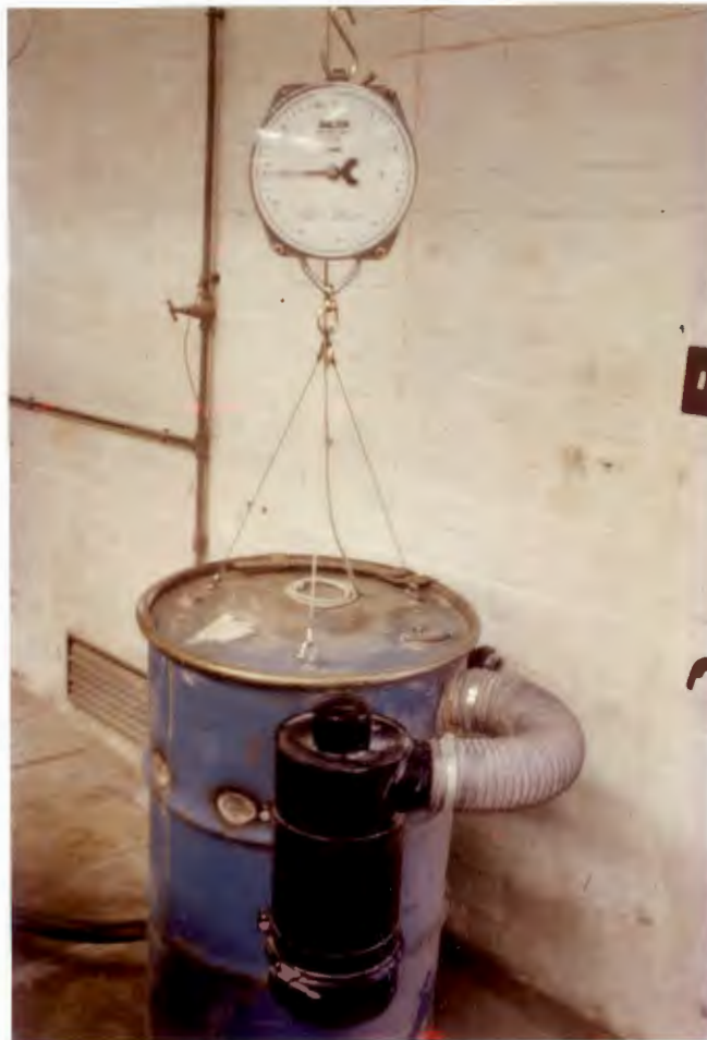
FIG: 3.12 Suspended ash trap to facilitate ash mass recording with air filter unit evident.
