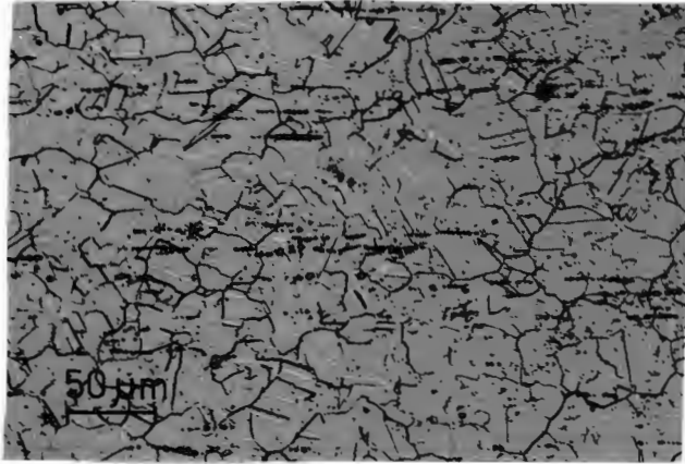
FIG : 4.13 Low magnification microstructure of 304 S/S test specimen showing sulphide stringer orientation (Oxalic acid).
