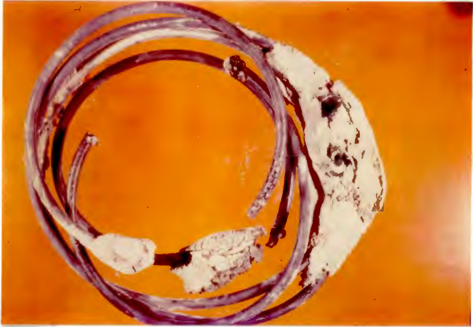
FIG: 3.17 Example of failed heater element sections with evidence of melting and fused ash.
