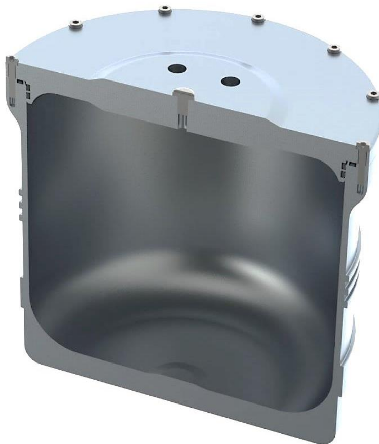
Figure C1: Rendering of a cross-section of the Power Pod housing
