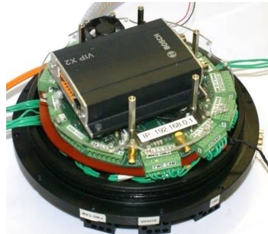
2. First shelf with video encoder & 1 st fan
