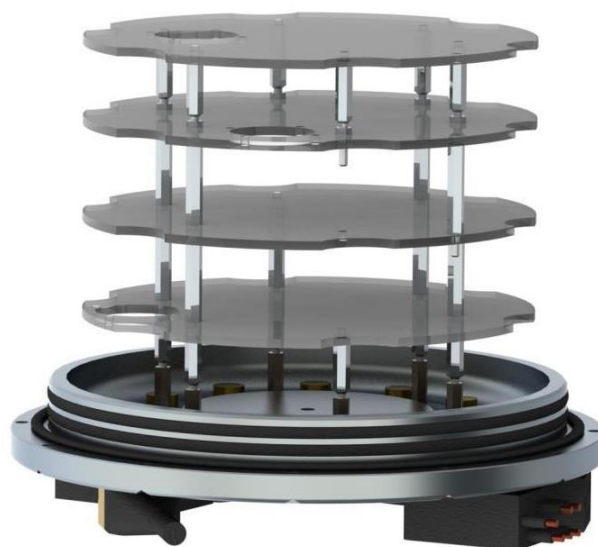
Figure 56: Rendering of the E-Pod "shelving" system mounted on the underside of the housing lid
