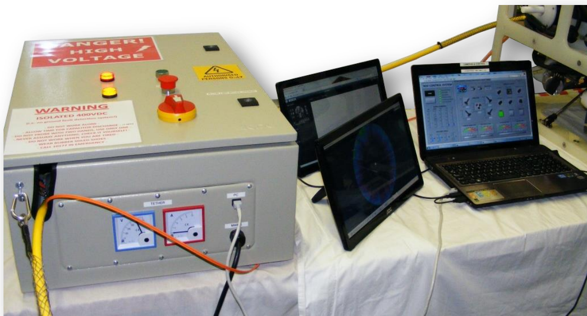
Figure 95: Photo of the surface control station with the PSU enclosure (left) and laptop with auxiliary screens displaying the user interface (right)
