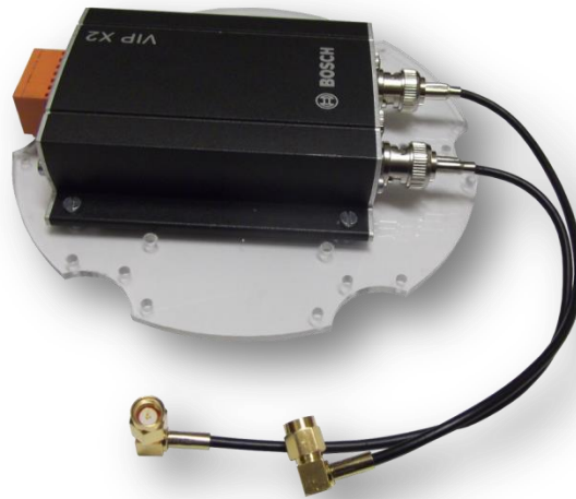
Figure 59: Photo of the Bosch VIP X2 video encoder mounted on its Perspex® shelf
