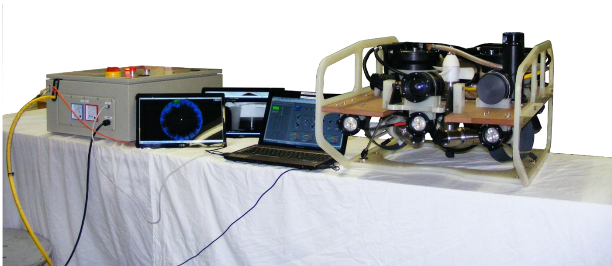
Figure 3: Photo of the ROV (without cover and float block) alongside the surface power supply and user interface
