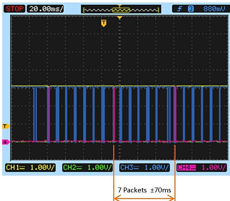
Figure 111: Oscilloscope screen capture showing the frequency of serial data packets (blue) and the frequency of each transmitted byte from the bottom E-Pod controller (magenta) when using the simplified user interface
