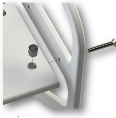
Figure 39: Fastener system used to join the ROV frames
