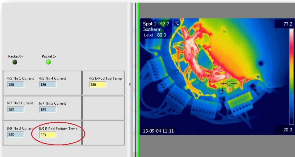
Figure D2: Screen capture of ADC readout in a Labview® User Interface and thermal reading of bottom E-Pod PCB temperature sensor in FLIR® IR Monitor software
