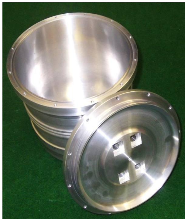
Figure 41: Photo of the Power Pod's aluminium housing
