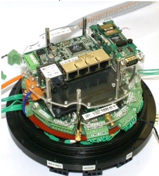
3. Second shelf with fibre optic switch & RS-485 Tibbo®
