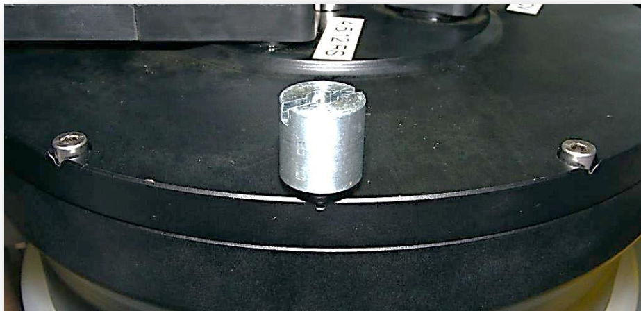
Figure C9: Zinc anode fitted to the Power Pod
