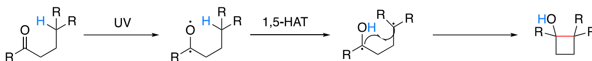
Scheme 4.7: General reaction scheme of Norrish-Yang photocyclisations via a 1,5-HAT from carbon to oxygen.
