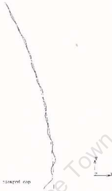
Figure 15: clamped cap, eigenmode 15, critical pressure 0.1526 N/mm 2
