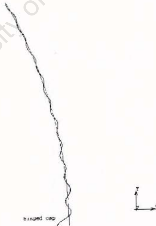
Figure 14: hinged cap, eigenmode 14, critical pressure 0.1374 N/mm 2
