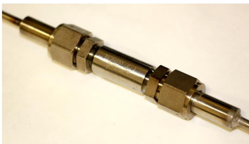
Figure 4.2: Photograph of tubular reactor used for OMCVD. Taken from Jackson, 2015.
