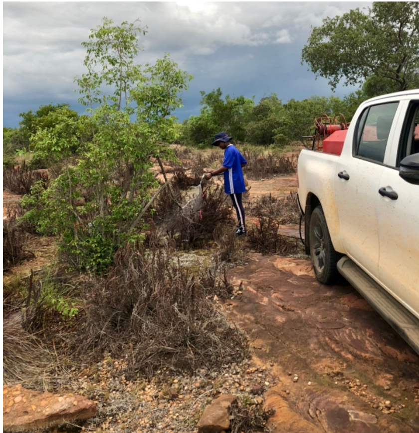
Figure 3-S1. Simulation of rainfall using a hose pipe connected to the portable fire water tank and a generator to rehydrate Myrothamnus flabellifolia plants in the Swebeswebe field site.
