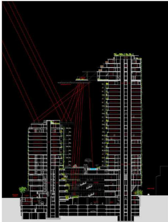
The red lines represent the sun rays being reflected by the mirrors (heliostats); this allows natural sunlight to be redirected into the courtyard below.
