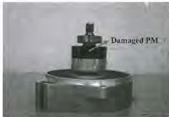
Figure 3.4: Implementation of the damaged PM fault
