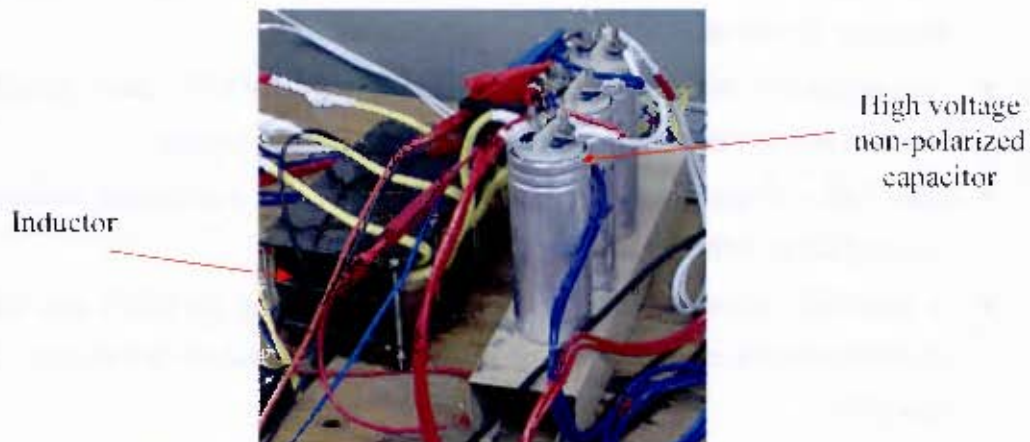
Photo 5.1.5-1: Low-pass filter inductor
