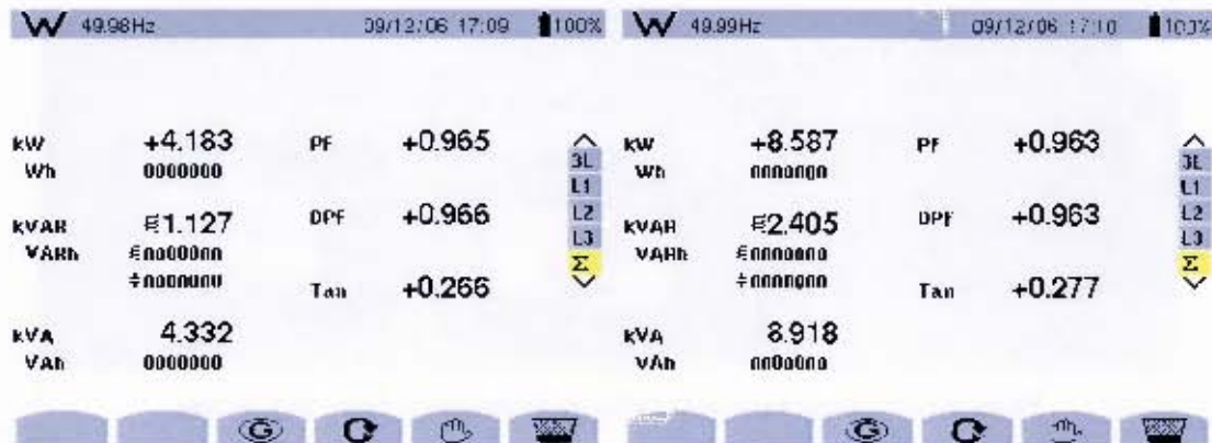
Power_Analyser_Result 5.1.2-1: Three-phase load capacity before and after closing S_{W2}
