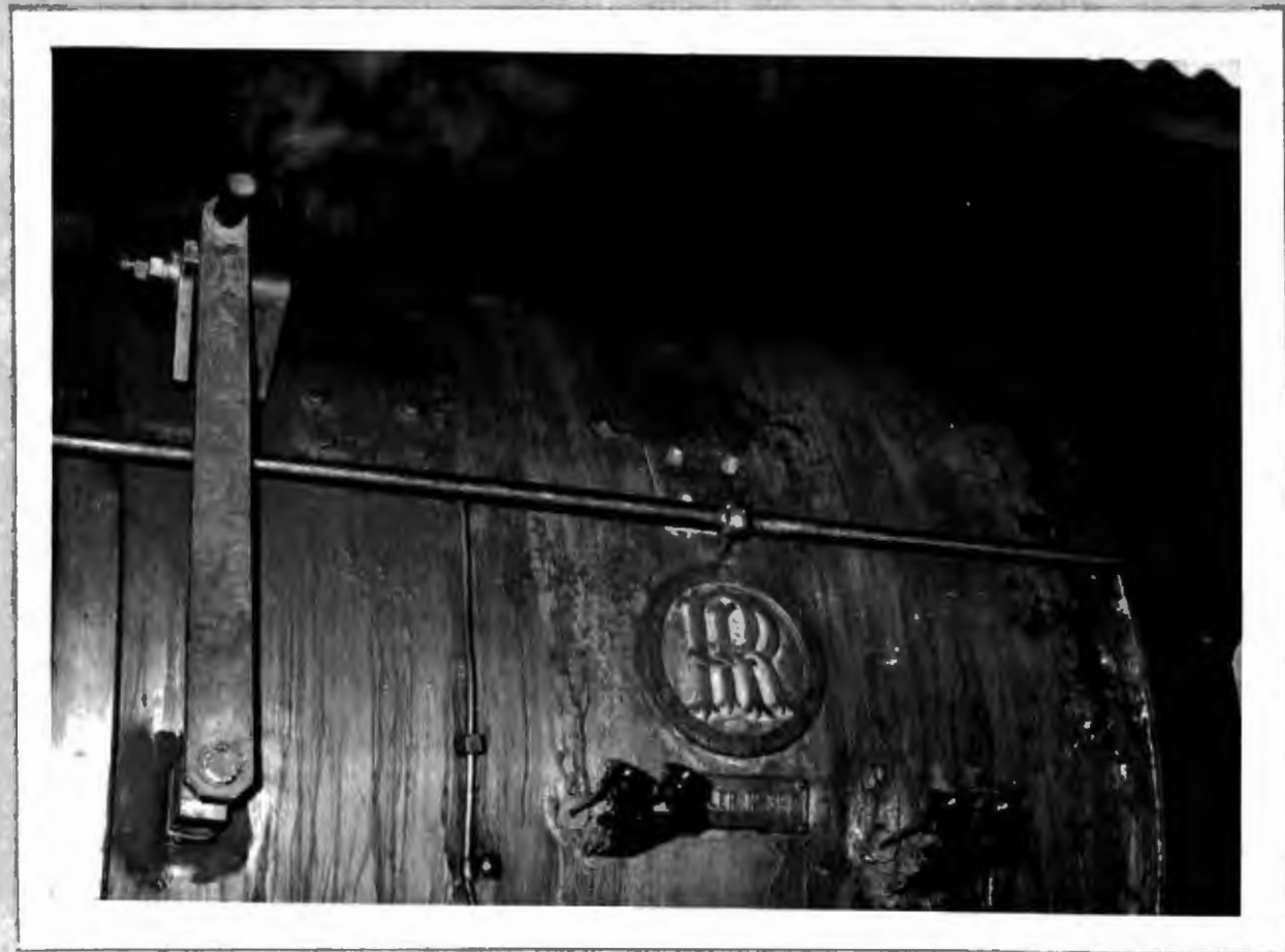
DAMPER LIFTING ARM; EXHAUST NOZZLE ADJUSTING SLIDE CONTROLS.
