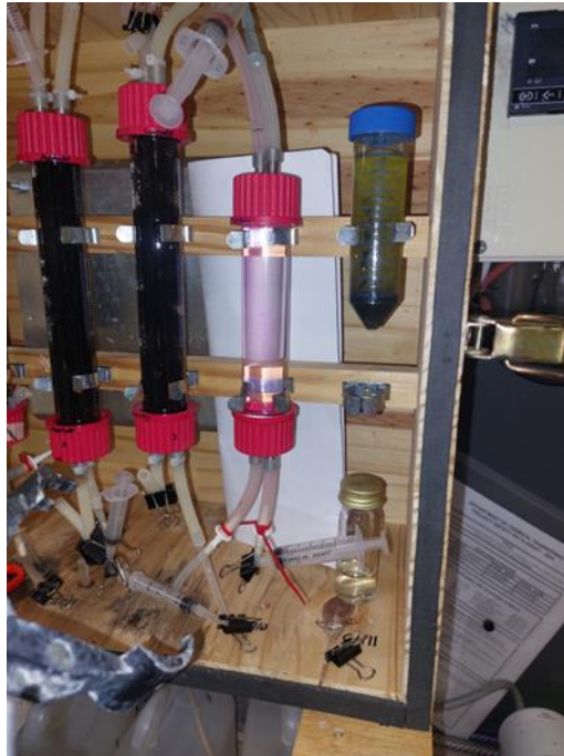
Figure 4-7: Mini column reactor at start-up of continuous operation with bulk liquid turned a faint pink from oxygen entering through the feed ports (dissolved oxygen test using resazurin dye)
