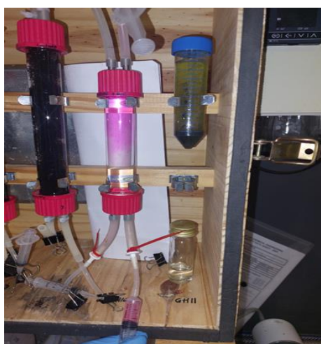
Figure 4-8: Sampling from the bottom of the mini-column reactor in continuous operation showing a colour change to pink from the top of the reactor (dissolved oxygen test using resazurin dye)
