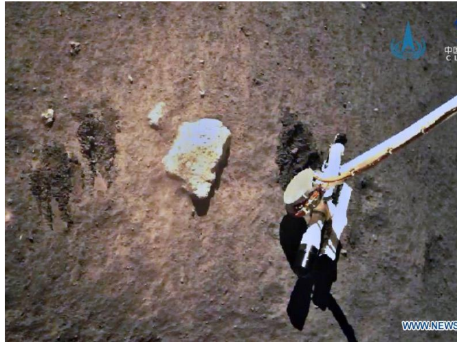
Figure 3-6: Picture of the Chang'e-5 probe gathering regolith samples on the Moon (Huaxia, 2022).
