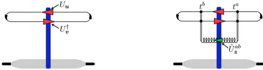
Figure 2.6: a) A dipole-target interaction. b) A dipole-target interaction in which the dipole emits a gluon, that passes through the target field and then gets reabsorbed by the dipole.
