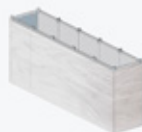
4) Shutter board fixed to Substructure
