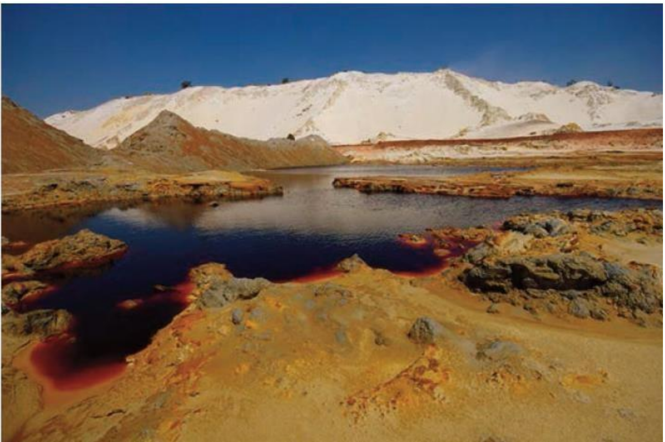
Figure 5. Acid mine drainage generated in surface tailings deposits in the West Rand (Coetzee, 2013).
