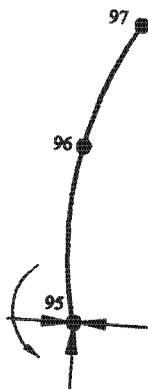
Fig. 5.3 Schematic drawing illustrating a node constrained in all direction.
