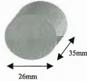
Fig.A.1: Physical dimensions of stainless-steel specimen.
