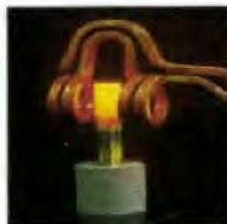
Figure 2.2: Through heating of a steel work-piece using a saddle coil [12].
