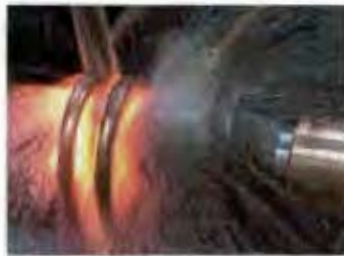
Figure 2.3: Surface heating by induction followed by a quench cycle [12].
