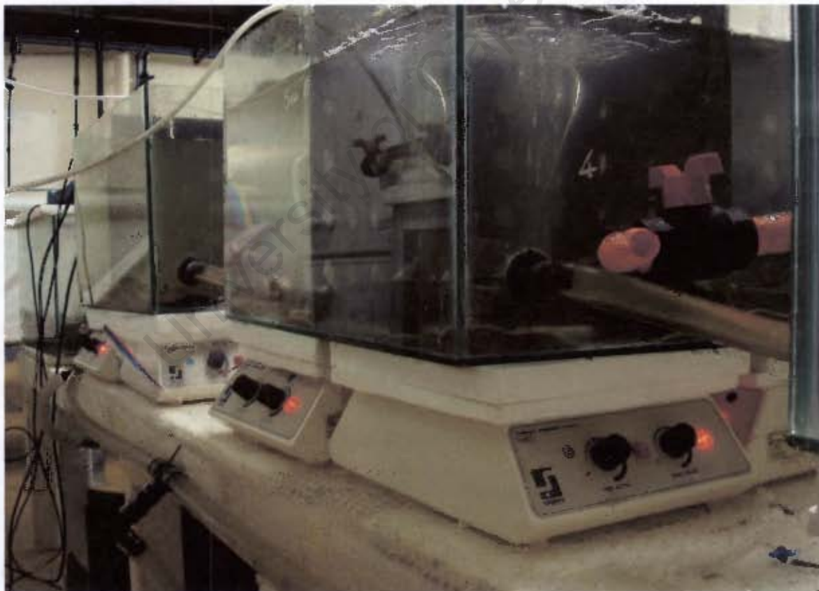
Figure 4.2: Two of the three medium-term experimental aquaria. The magnetic stirrers and the polystyrene support between the aquaria and the stirrers are also shown.
