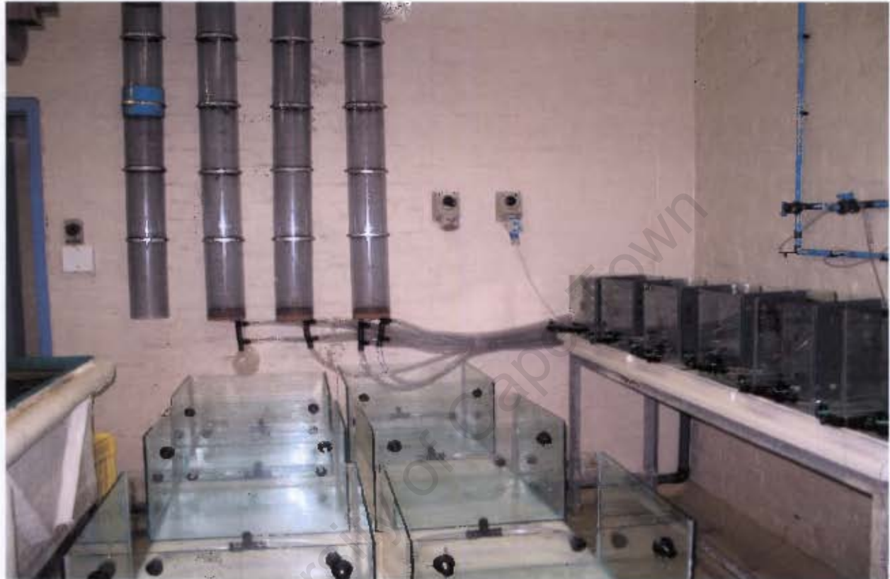
Figure 3.2: Gas experimental setup during the initial stages of construction. The six short-term aquaria are visible on the right hand side while the aquaria used in the turbidity experiments described in Chapter 4 are in the centre. The four Perspex gas-regulation cylinders are mounted on the wall. All the short-term tanks already have the regulation valves attached and the first two short-term tanks are connected to the nitrogen-stocking cylinder on the right. The short-term tanks already have single grey PVC separators installed.
