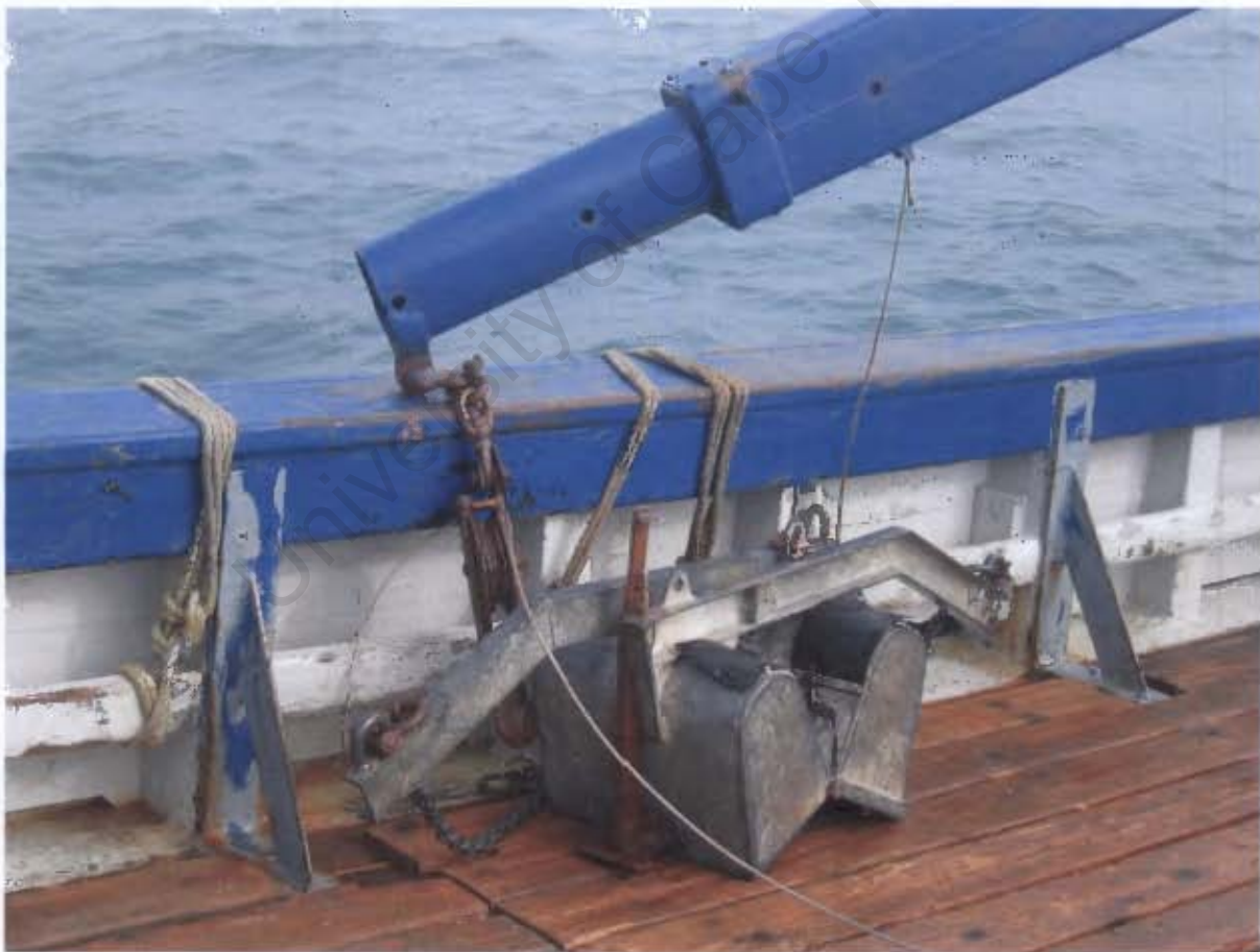
Figure 4.1: The Van Veen grab sampler (grey) and crane (blue) used for the sediment sampling.
