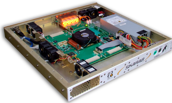
Figure 3.8: Figure showing the SKARAB processing node. Image source: [32]
