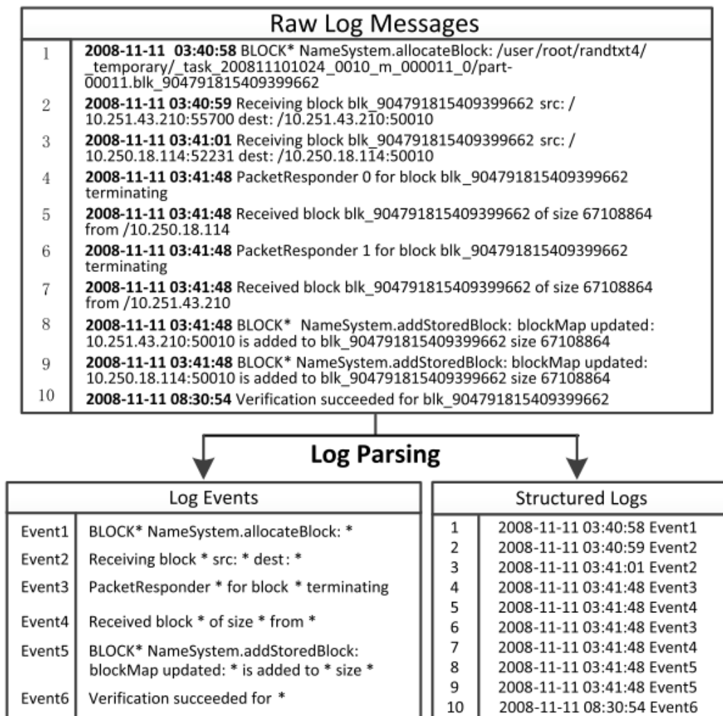
Figure 3.12: Figure showing raw logs being parsed into a event templates and arranges as a sequence of event templates. Image source: [35]
