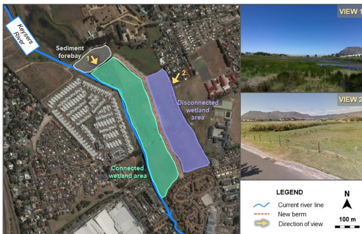
Figure 6-7: Configuration of the modelled Dreyersdal wetland upgrade (Plan view: Bing Maps, 2021; View 2: Google Maps, 2021)
