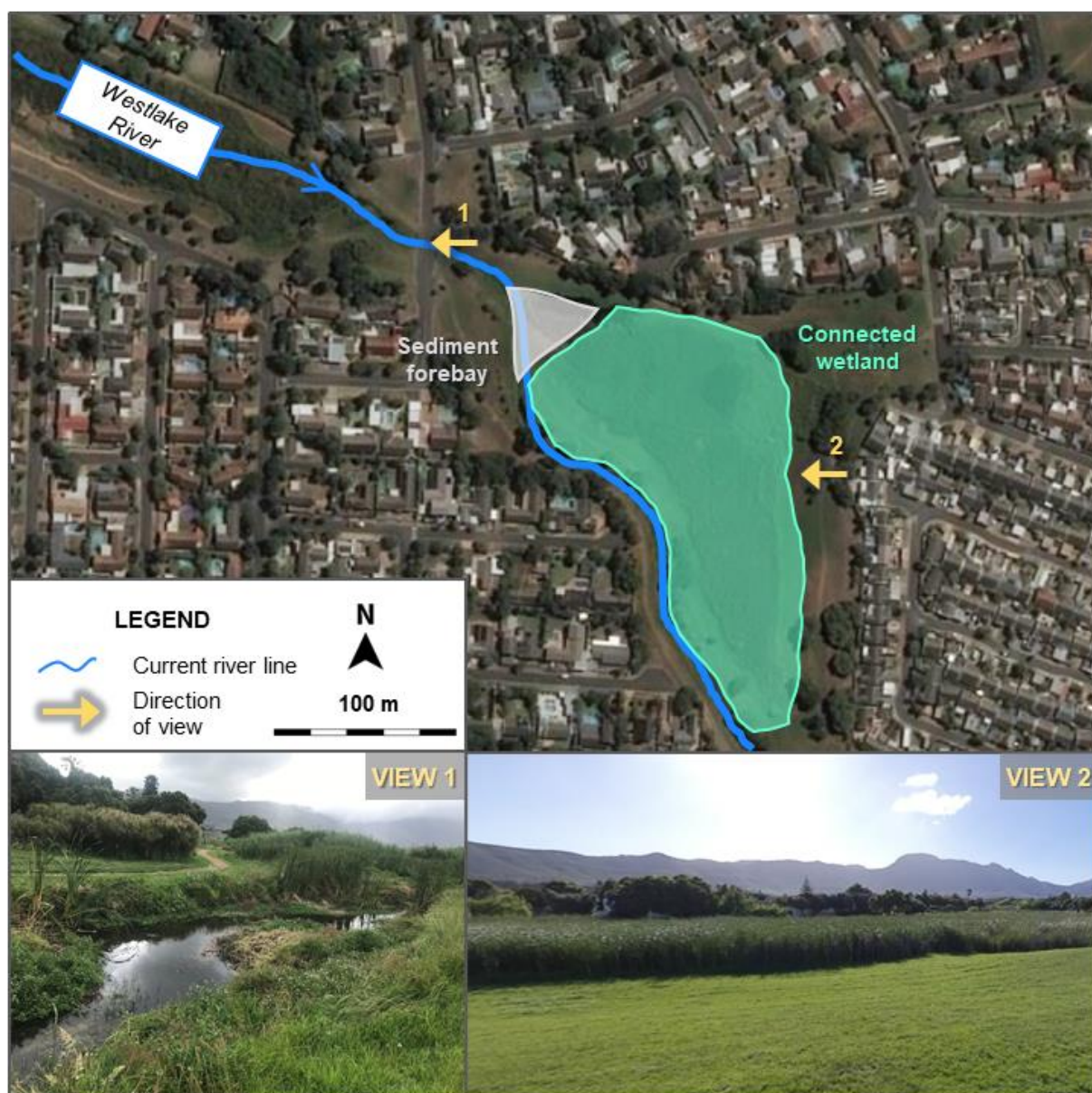
Figure 6-15: Configuration of the modelled Kirstenhof Greenbelt wetland upgrade (Plan view: Bing Maps, 2021; View 2: Sean Paterson, 2019)
