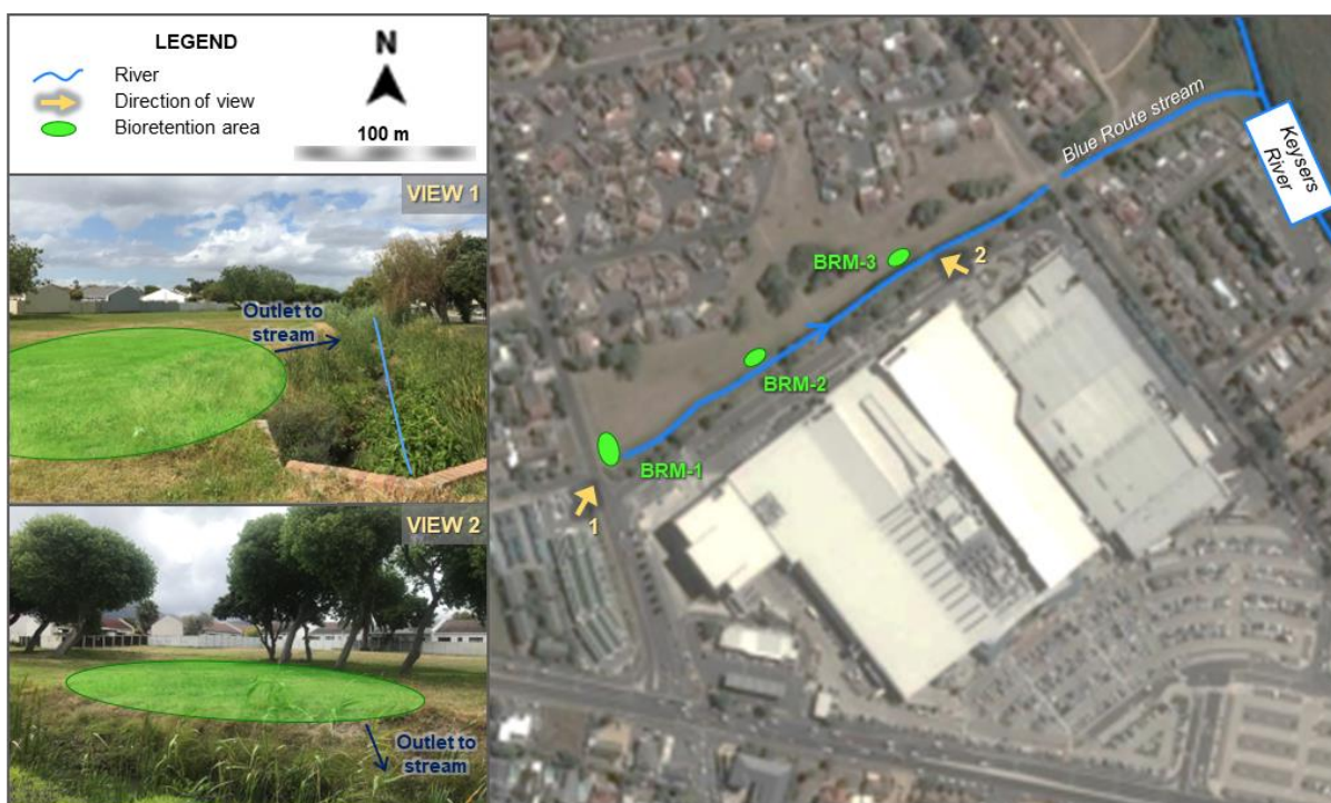
Figure 6-10: Modelled bioretention areas behind Blue Route Mall (Plan view: Bing Maps, 2021)
