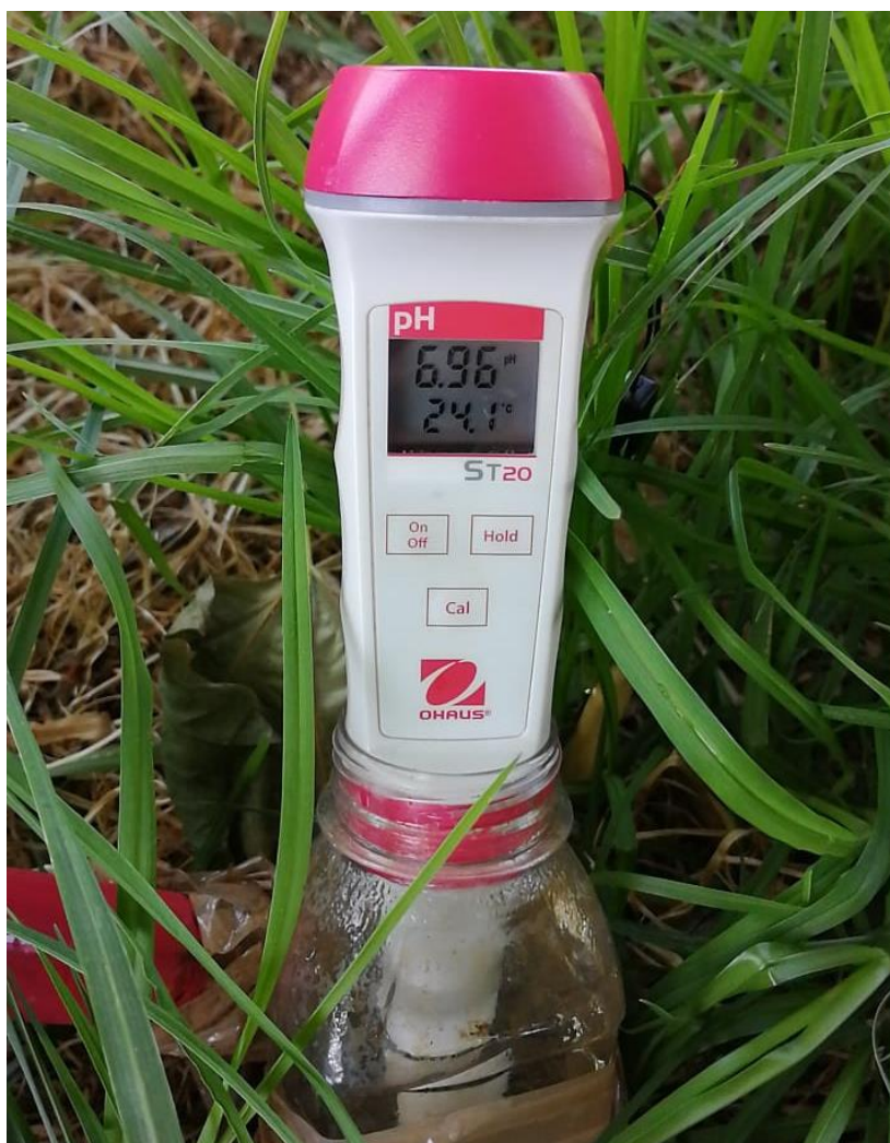
Figure 4-2: A portable pH pen meter taking a reading in a sample bottle
