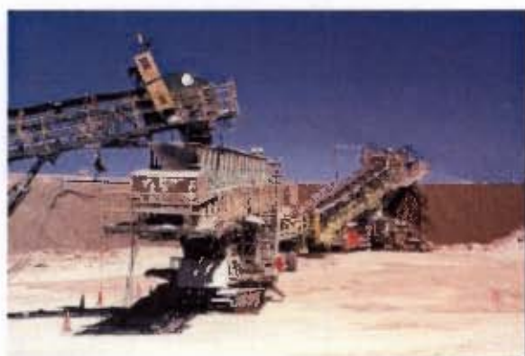
Figure 3.2: The sociedad minera cerro verde s.a.a., Arequipa, Peru; Crushed, agglomerated, ore conveyed to stacker (Hansford, 2005) presented at IBS'05, Cape Town
