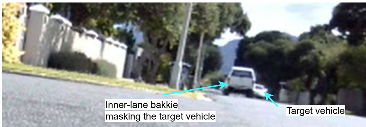
Figure A.3: Video frame of the target masking during the 48 km/h controlled test
