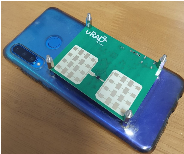
Figure 6.5: Photograph of the uRAD USB v1.2 and phone camera test rig
